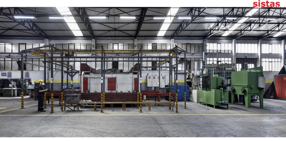
Heat Treatment demands of our customers are in our Ipsen chamber furnace, annealing furnaces and suppliers being carried out. Applied processes: - Breeding - Cementation - Soft Annealing - Normalization - Isothermic Annealing - Stress Relief Annealing - Induction Hardening In addition, controlled cooling process for microalloyed steels is applied with automatic cooling conveyors.
